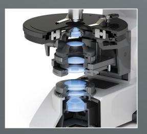
For precise conoscopic imaging, an integrated module with focusable Bertrand Lens is provided between the viewing body and the specimen. Centration of the Bertrand Lens is achieved through easily accessible centering screws. Parking slots are built into the analyzer module for convenient storage of allen key drivers that facilitate centering of the analyzer and the objectives.
